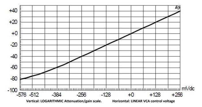
On this VCA-2162 module, volumes (or better: attenuation/gain) of both channels are set separately by 0-4,8Vdc LINEAR control signals, f.e. coming from a regular, mechanical LINEAR potentiometer(s). Use a single potentiometer and tie both control inputs to this if there is no balance function required.
