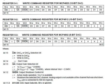
The MCP4802, 2-channel, 8-bit DAC as we use here, is controlling both VCA channels separately and need to be programmed separately as well. Data will only be accepted while the CS pin is low. Only after data is latched, the DAC and the output amplifier will come alive. Till that time the output pin is grounded by a 500kohm resistor. Note that redundant data bits, used for higher resolution DAC's will be ignored.
